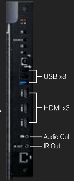
Onboard in/out control panel
